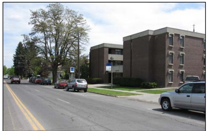
Current parallel parking along Sharp could be considered for “back-in” angled parking as a means of increasing the number of on-street stalls in the area.
